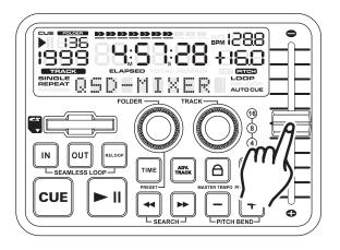
**Using the Pitch slider (26):** Be sure the pitch function has been engaged as described above. To use the *PITCH SLIDER (26)* slide the slider up and down. Down will increase the pitch and up will decrease the pitch.
